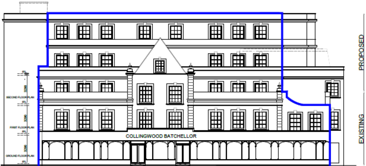
SOUTH WEST ELEVATION (facade on Victoria Road)
