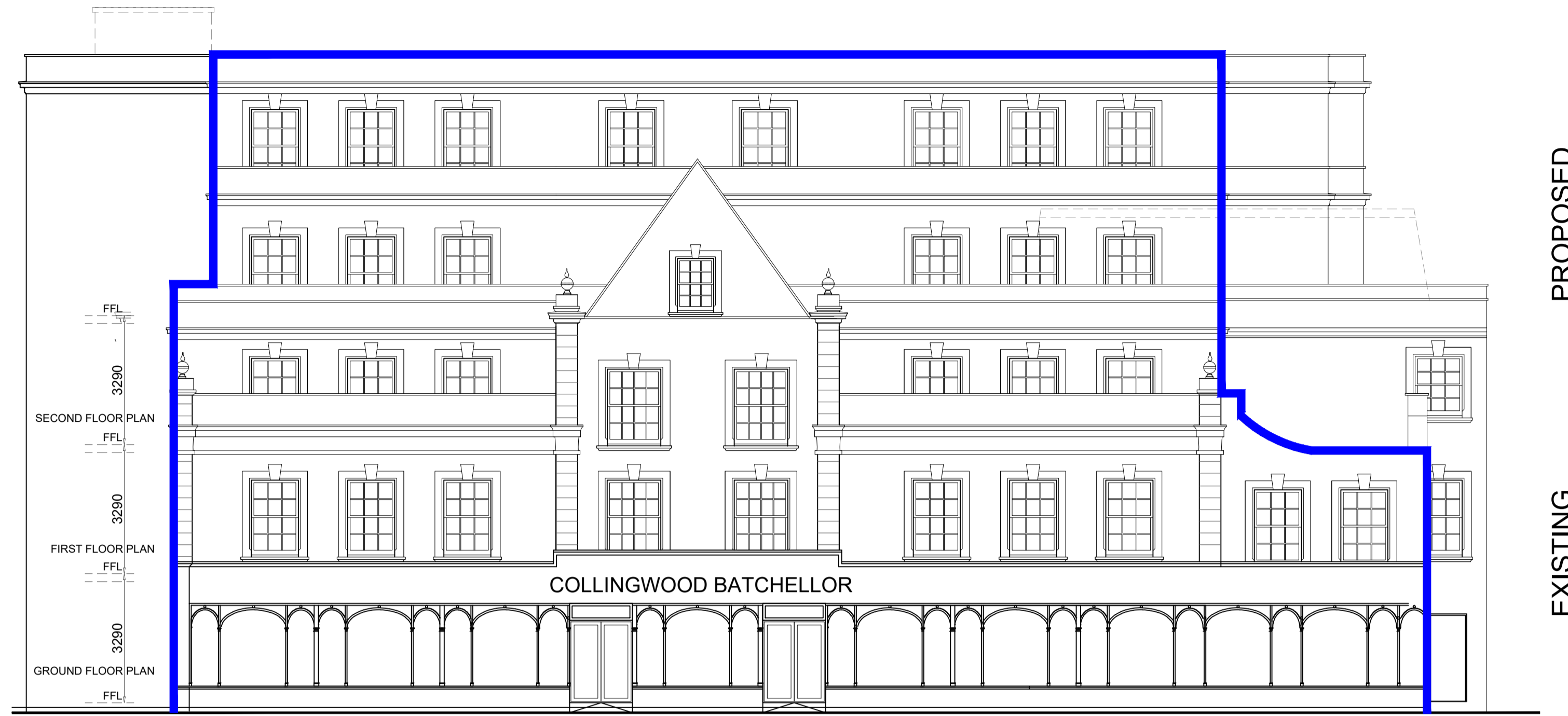
SOUTH WEST ELEVATION (facade on Victoria Road)
